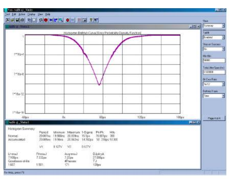
Figure 10. Bathtub Curve showing failing spec
